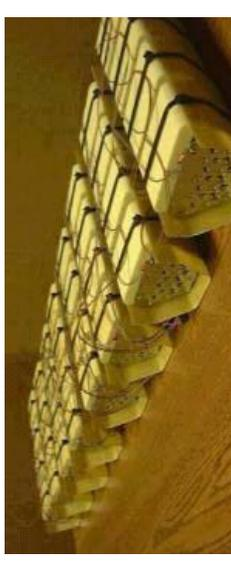
**Option C** Multy cell 48V lithium packs, one for each of the dc/dc converters
