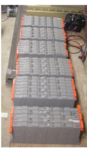
**Option B** groups of 7 Prius NIMH subpacks will make up a 6.5AH boost pack, one for each dc/dc converter. Total of 70 subpacks, or 420 cells
