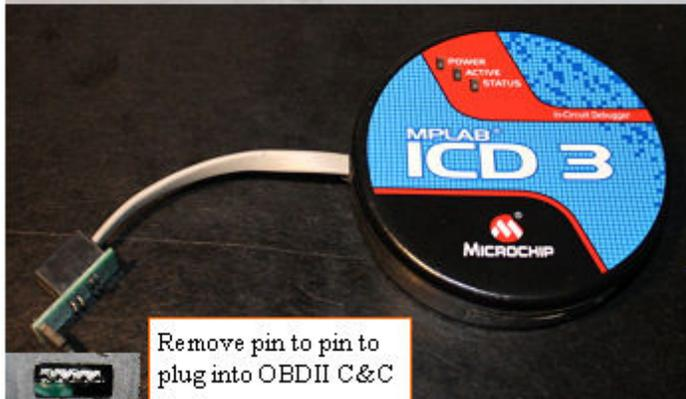
Remove pin to pin to plug into OBDII C&C
