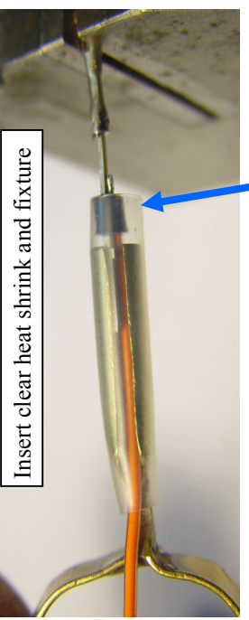
Shrink clear end at black heat shrink area After it cools slide out the fixture
