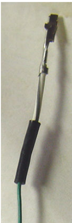
Normal crimp on 22ga wire soldered to ribbon wire and heat shrink
