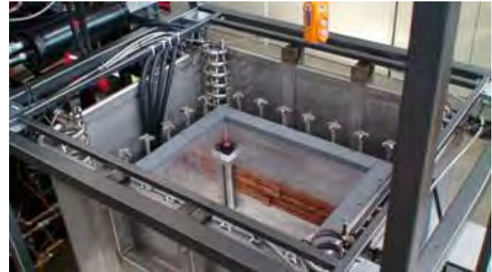
Calorimeter test chamber in isothermal fluid tank
