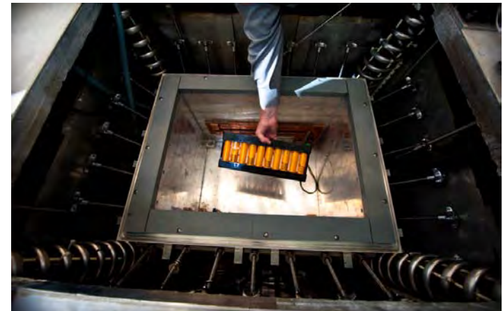
Top view of calorimeter test chamber
